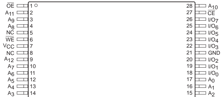
TSOP Top View (8mm x 13.4mm) (T13)
