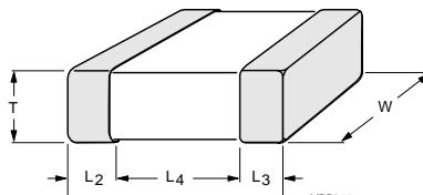
Fig. 2 Surface mounted multilayer ceramic c
