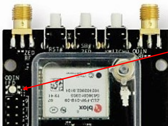
Figure 8: ODIN-W2 activity LED position on C099-F9P board
