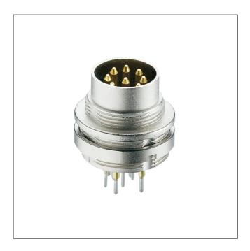
Chassis plug acc. to AISG specification and IEC 61076-2-106, IP 68, with threaded joint, for printed circuit boards, for front mounting
