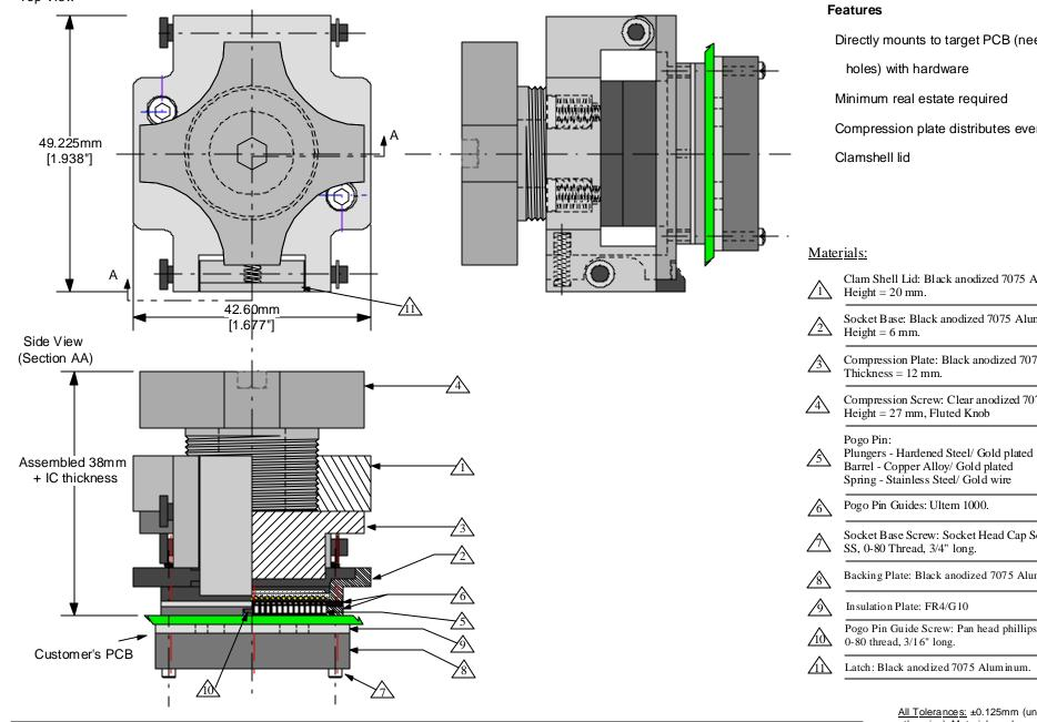
Directly mounts to target PCB (needs tooling
