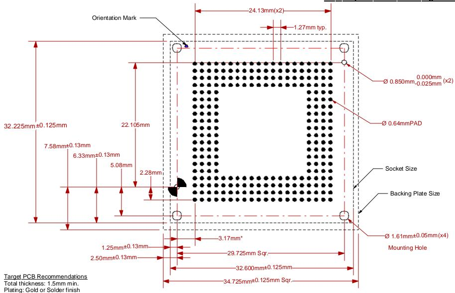
Recommended PCB Layout Tolerances: ±0.025mm [±0.001"] unless stated otherwise.
