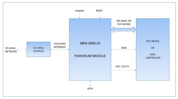
This block diagram present the 0804-5000-25 powerline module in a typical environment. Seven different types of interfaces are shown. These interfaces are described in detail below.
