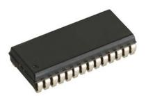
The device provides B3ZS (DS3) or HDB3 (E3) encoding functions for data to be transmitted to the line. A complimentary decoder circuit is also included in the chip for decoding received signals from an external line receiver. Both encoder and decoder functions can be disabled independently through external control pins. In the receive direction, coding errors and bipolar violations are detected and flagged at an output pin.
