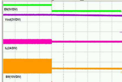
Shutdown Through Enable_no load
