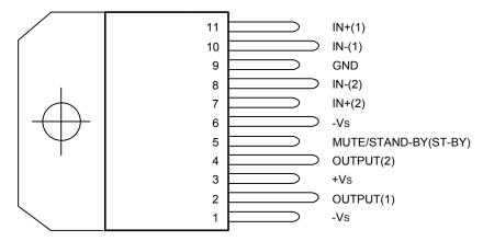
\* TAB CONNECTED TO PIN 6
