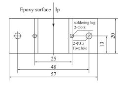
Noted:Welding needle is used in model FZ. Soldering lug is used in model FP. Model FL is leading cable from the soldering lug.
