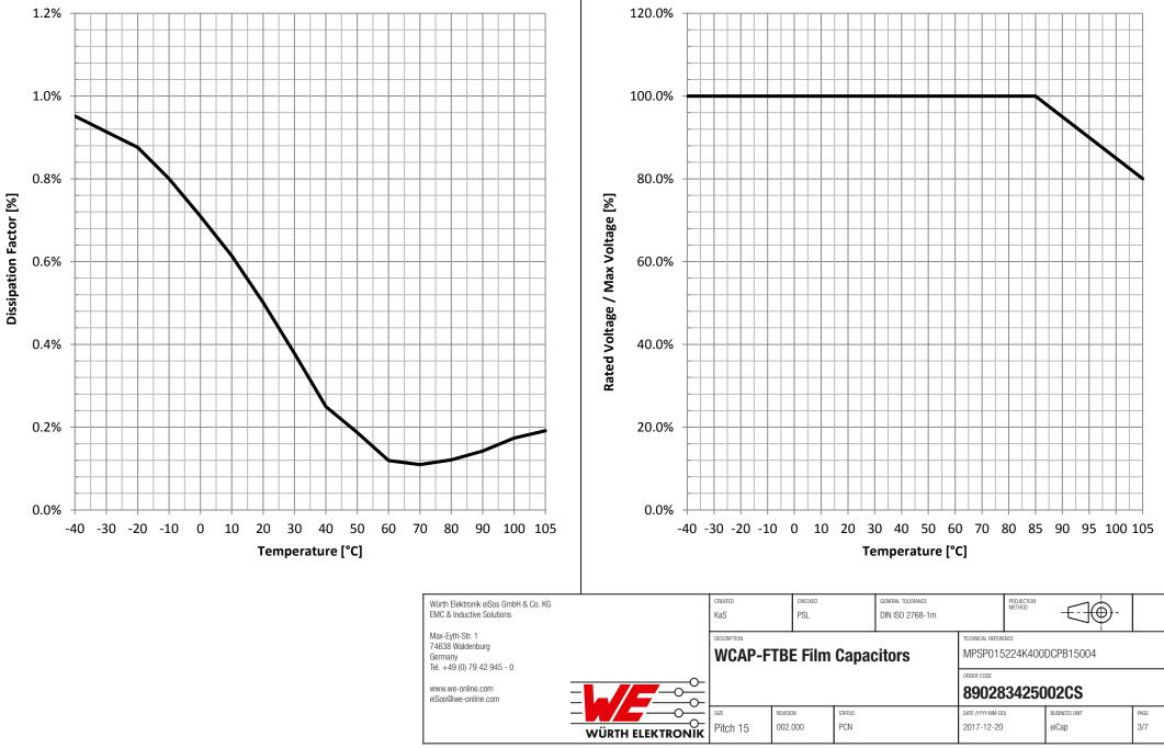
**Rated Voltage vs. Temperature:**
