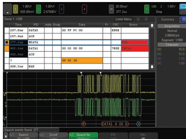
Figure 21. USB 2.0 trigger, decode and "lister" display.
