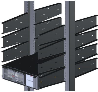
FIGURE. 5: INSTALL FIRST T1000 MODULE
