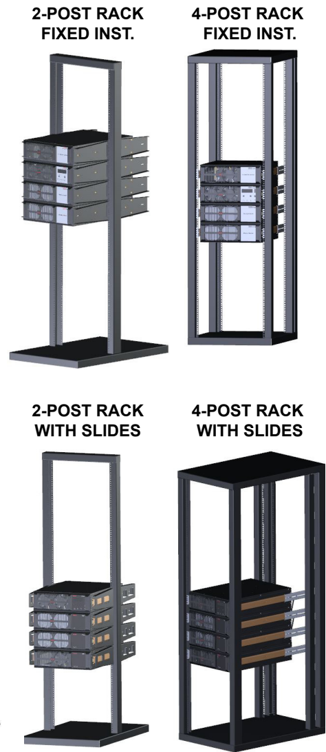
FIGURE 6-6: RACK INSTALLATION OPTIONS
