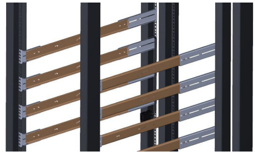
FIGURE 7: INSTALL REMAINING SLIDE RAIL ASSEMBLIES IN 4-POST RACK
