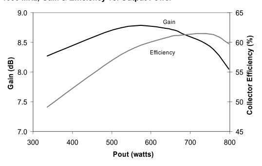
RF Power Transfer Curve 1090 MHz, Gain & Efficiency vs. Output Power
