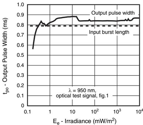
Fig. 2 - Pulse Length and Sensitivity in Dark Ambient
