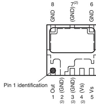
Proposed pad layout from component side (dim. for reference only)
