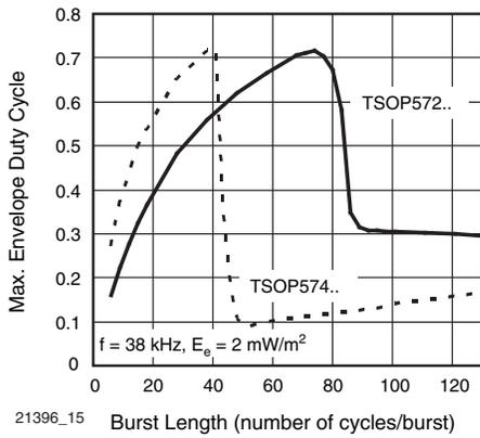
Fig. 8 - Max. Envelope Duty Cycle vs. Burst Length
