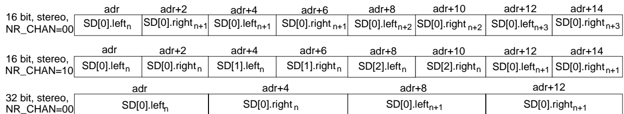
Figure 2: Examples of Audio Out Memory DMA Formats
