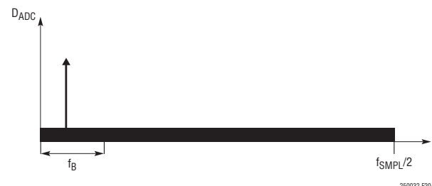
Figure 20. Frequency Spectrum of SAR ADC Core Output
