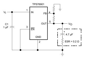
Figure 6. Typical Application Circuit
