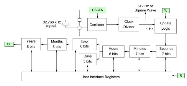
Figure 7. Real-time Clock Core Block Diagram
