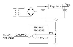
The voltage on the PFI input pin is compared to an onboard 1.2 V reference. When the PFI input voltage drops below this threshold, the comparator will drive the CAL/PFO pin to a LOW state. The comparator has 100 mV (max) of hysteresis to reduce noise sensitivity, only for a rising PFI signal. For a falling PFI edge, there is no hysteresis.
