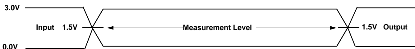
Figure 17. Input Waveforms and Measurement Levels
