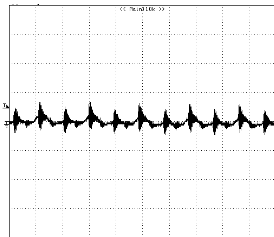
Figure 14: Output voltage ripple at nominal input voltage and rated load current ( I_o=40\text{A} ) ( 20\text{ mV/div} , 2\mu\text{s/div} ) Load capacitance: 1\mu\text{F} ceramic capacitor and 10\mu\text{F} tantalum capacitor. Bandwidth: 20\text{ MHz} . Scope measurements should be made using a BNC cable (length shorter than 20 inches). Position the load between 51 mm to 76 mm (2 inches to 3 inches) from the module.
