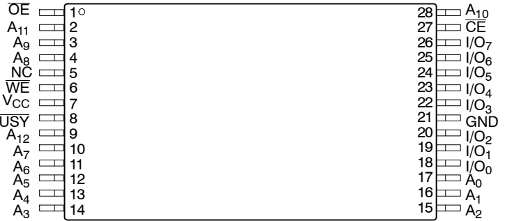
TSOP Package (8 mm x 13.4 mm) (H13)
