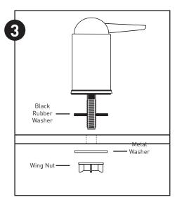
(C) From under the sink, slide the metal washer on and thread on the wing nut. Tighten the wing nut by hand until tight. It may be necessary to have a second person to hold the faucet while tightening the wing nut.
