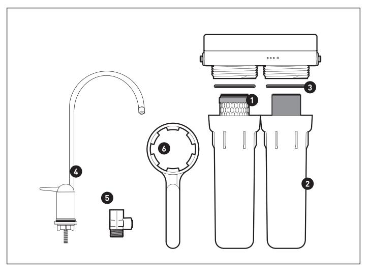
If flow through empty system is adequate, place one filter cartridge in system at a time and check flow to make sure cartridge is not clogged. Replace clogged cartridge if necessary.
