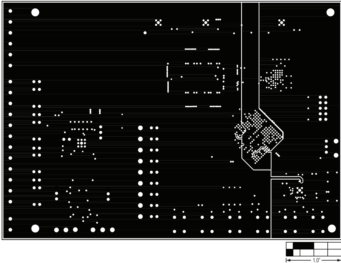
Figure 17. MAX11043 EV Kit PCB Layout—Signal Layer 6
