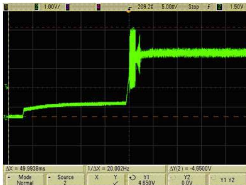
Figure 8. Input Voltage Overshoot >4V (Bad)
