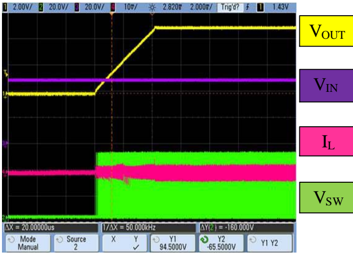
Figure 25. Start-Up Transition at No Load (EN = High)
