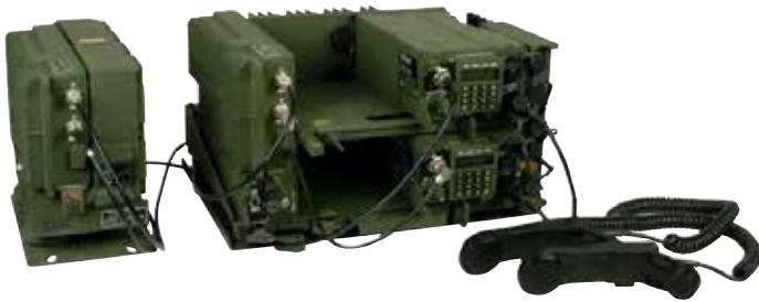
RT-1523 in a VAA mount, 50 W dual long range (retransmit), plus 2nd power amp and retrans cable
