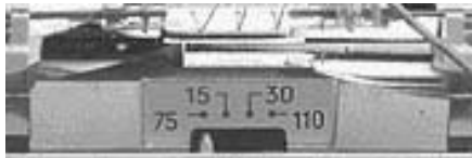
Multi-Candela Indicator (bottom of Strobe Lens)
