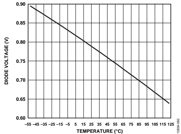
Figure 82. Temperature Diode Voltage vs. Temperature
