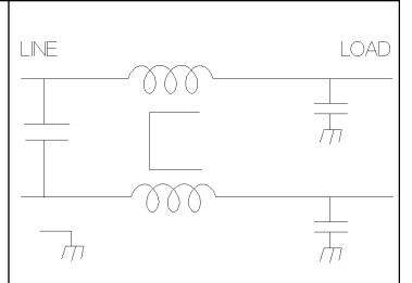
Diel. Withstanding (Line—GND) = \_\_\_\_\_1500 VDC; 1 Min Diel. Withstanding (Line—Line) = \_\_\_\_\_1500 VDC; 1 Min
