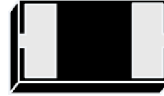
DFN1006-2L (Bottom View)
