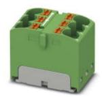
Distribution block, bridged internally, nom. voltage: 630 V, nominal current: 32 A, connection method: Push-in connection, number of connections: 6, cross section: 0.2 mm² - 6 mm², AWG: 24 - 10, width: 18.5 mm, height: 21.7 mm, color: green, mounting type: NS 35/7,5, NS 35/15
