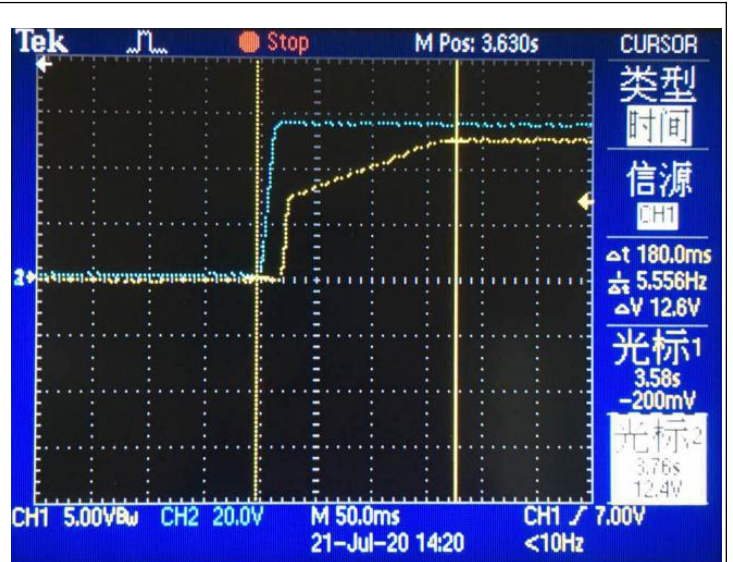
Output response & load (12V / 0.02A)
