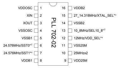
Note: 25MHzx2: double drive strength <sup>v</sup>: Internal pull-down resistor (120kΩ)
