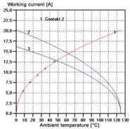
1 Temperature rise 2 Derating 3 Derating curve at I max \* 0,8 (DIN IEC 512)
