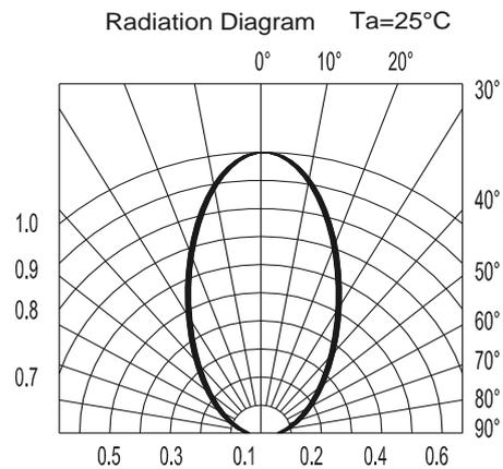
Typical Electro-Optical Characteristics Curves
