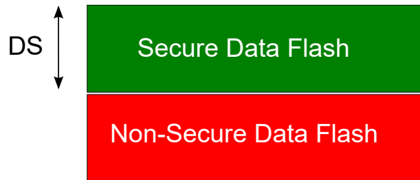
Figure 13-3. SAM L11 Data Flash Memory Mapping
