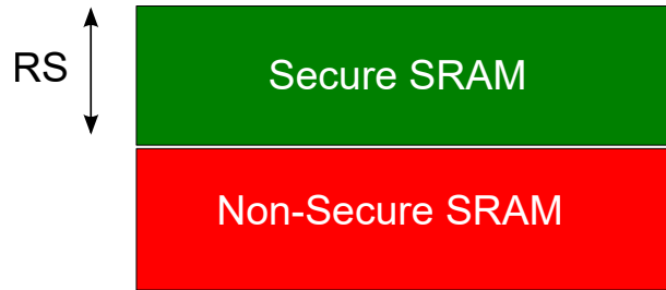
Figure 13-4. SAM L11 SRAM Memory Mapping
