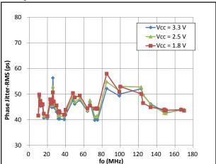
Phase Jitter RMS (Integration bandwidth 1.8 M to 20 MHz)
