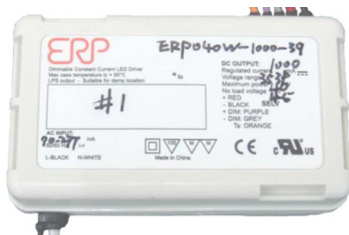
Figure 4: CXA2530 retail track light driver
