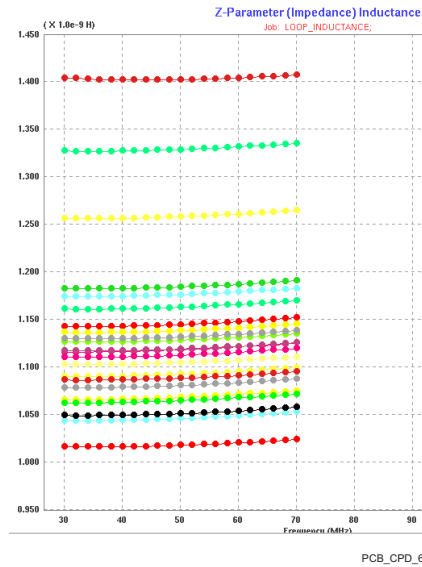
Figure 8-26. vdd_mpu Decoupling Cap Loop Inductances
