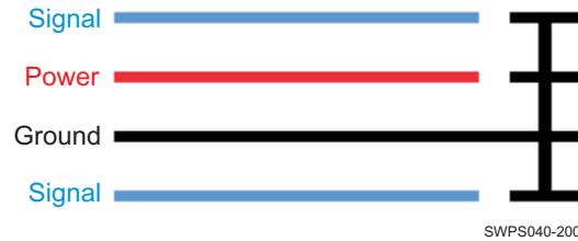
Figure 8-19. Guard Ring Routing
