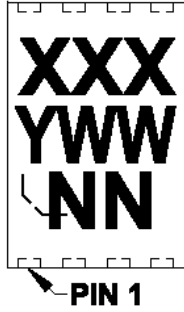
8 引脚 TDFN (2x3x0.75 mm) (MCP6V12)
