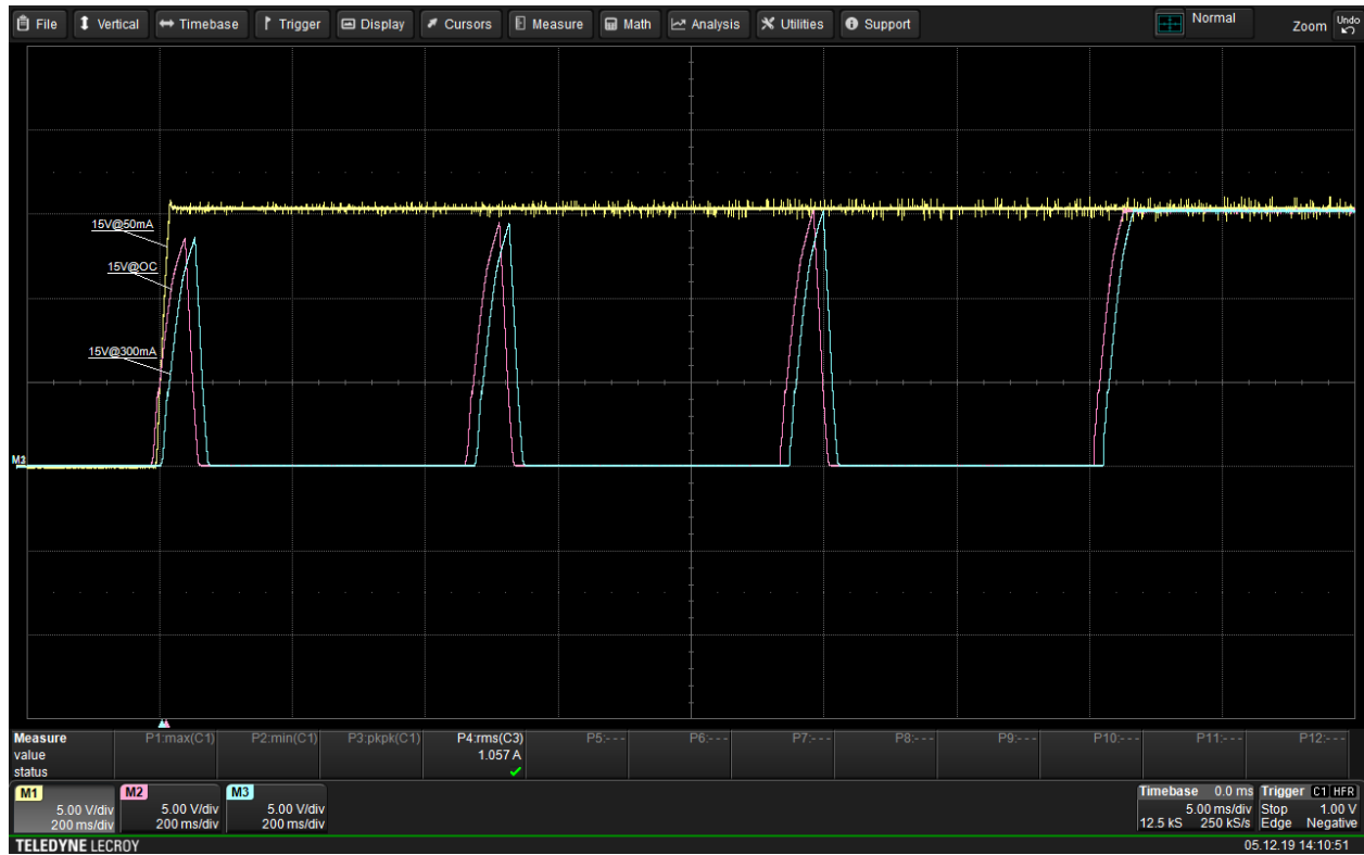
Figure 15. Start Up to Open Circuit, to 50 mA and to 300 mA at 390 V DC Input
