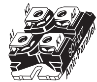
ISOTOP®[J] SOT-227 Antiparallel Configuration (ISOLATED BASE)
