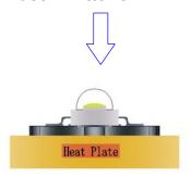
Put MCPCB on Heat Plate until Solder Paste melt. Put Emitter on MCPCB. Take the MCPCB out The Solder Paste sould be melted within 10 seconds. from Heat Plate within 10 seconds. Take out MCPCB out from Heat Plate within 10 seconds.
