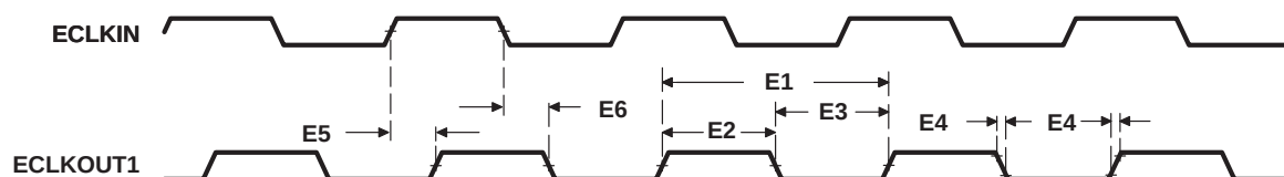
Figure 5–6. ECLKOUT1 Timings for EMIF Module
