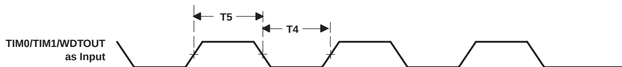
Figure 5–28. TIM0/TIM1/WDTOU Timings When Configured as Timer Input Pins
