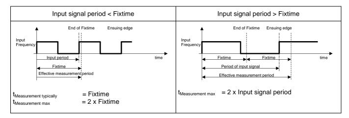
The total measurement time has a resolution of  $\pm$  0.4  $\mu s$ .
