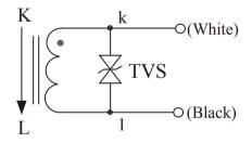
TVS: Transient voltage suppressor, Current output type
