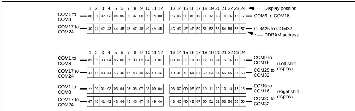
Figure 5 2-Line by 24-Character Display (5-Dot Font Width)
