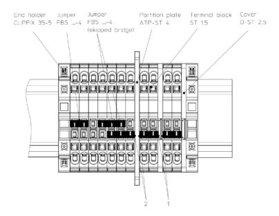
Depending on the separating plate between directly facing plug-in bridges, the rated voltages reduces to
