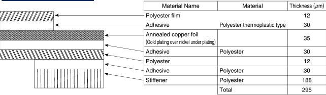
\* Actual tolerance of the thickness is approximately  $\pm 20 \mu m$ .
