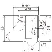
Note 1>: The coplanarity of each terminal lead within specified dimension is 0.1mm Max.
